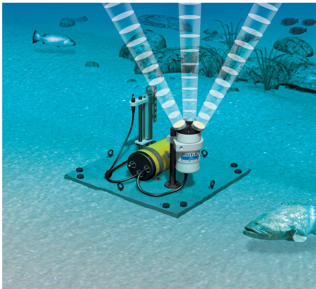
**Slika 4. ADCP (Acoustic Current Doppler Profiler) [7]**
