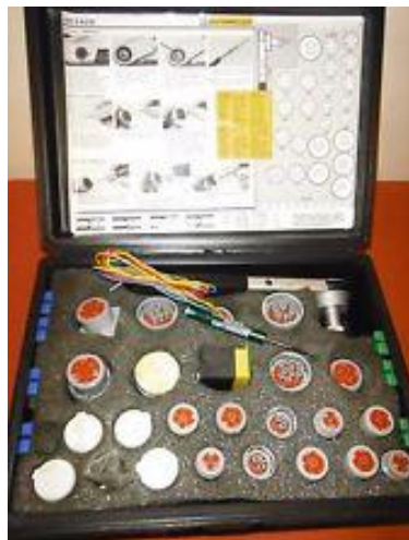
Slika 16. Caterpillarov indikator temperature [2]
