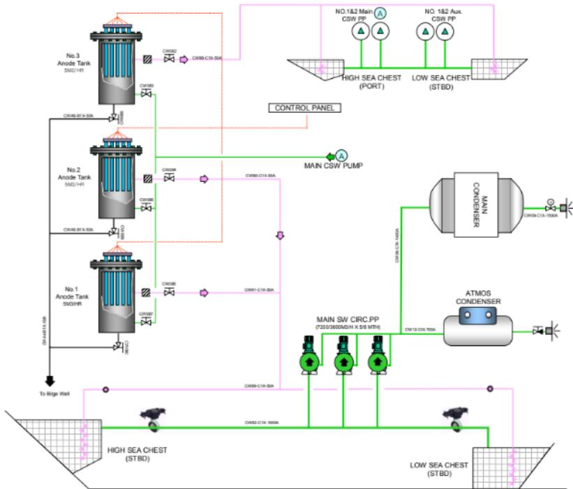
**Slika 9. Shema Marine Growth Preventing System (MGPS) [27]**
