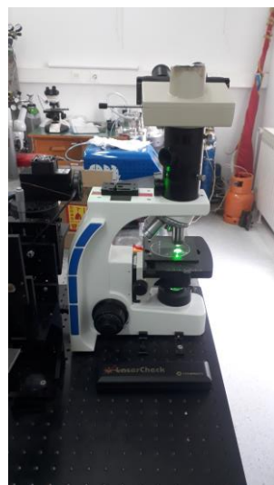
Figure 13. Standard optical microscope AMDSP XUM102 used for microscopic analysis of the samples with the prototype.
