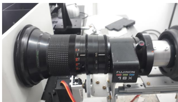
Figure 16. The Fujinon Lynx II A18x8.5, 1:1.7/8.5-153 mm attached to a spectrometer exit.
