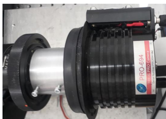
Figure 17. Optical sensor Trius PRO-694 monochromatic CCD mounted on the Fujinon zoom lens.
