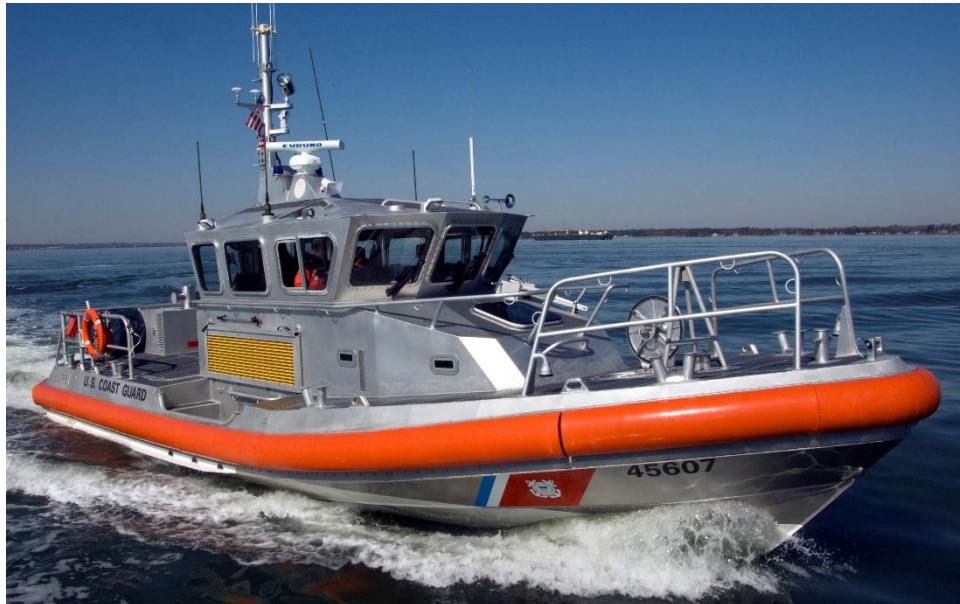
Slika 3. USCG 45ft (14 m), Response Boat Medium (RB-M) [11]
