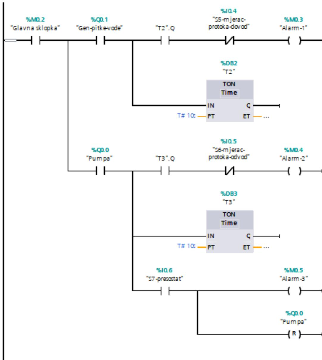
**Network 3: RESETIRANJE SVIH STANJA SENZORA**
